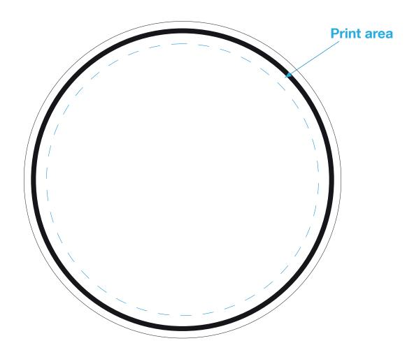
The registration movement is 2 to 3 mm per color in any direction There will be a thin line on the edge of the coaster in one of your printed colors
