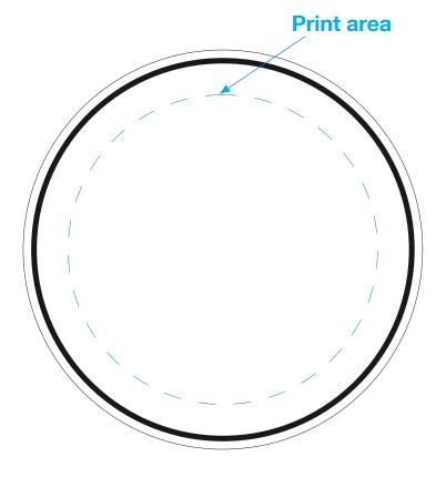
The registration movement is 2 to 3 mm per color in any direction
