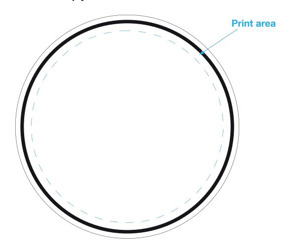
The registration movement is 2 to 3 mm per color in any direction
